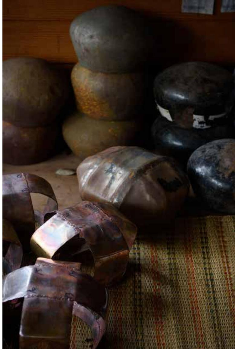
Ban Bat's alms bowl is famous because the community persists with an age-old method of crafting the bowls from slabs of steel using their hands and a hammer. The work requires laborious works from various artisans in each of the process – from making the rim, putting the pieces together, blowing, designing, hammering, and filing. Expertise and tremendous amount of effort are needed. Making one piece of alms bowl takes several days to complete.
